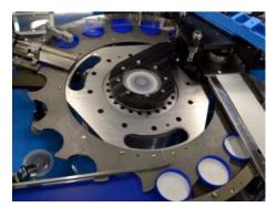
One assembly machine, able to process closures having very different dimensions. Flexibility, reliability and high speed are the key words featuring the latest solution from Gefit. This "lining machine" recently developed by the Italian company presents many innovations, that will certainly draw the attention of all manufacturers of closures with liner, from the food and beverage to the cosmetics industries.
